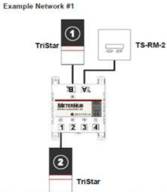
Figure 3-2. A simple two TriStar system with Remote Meter.
